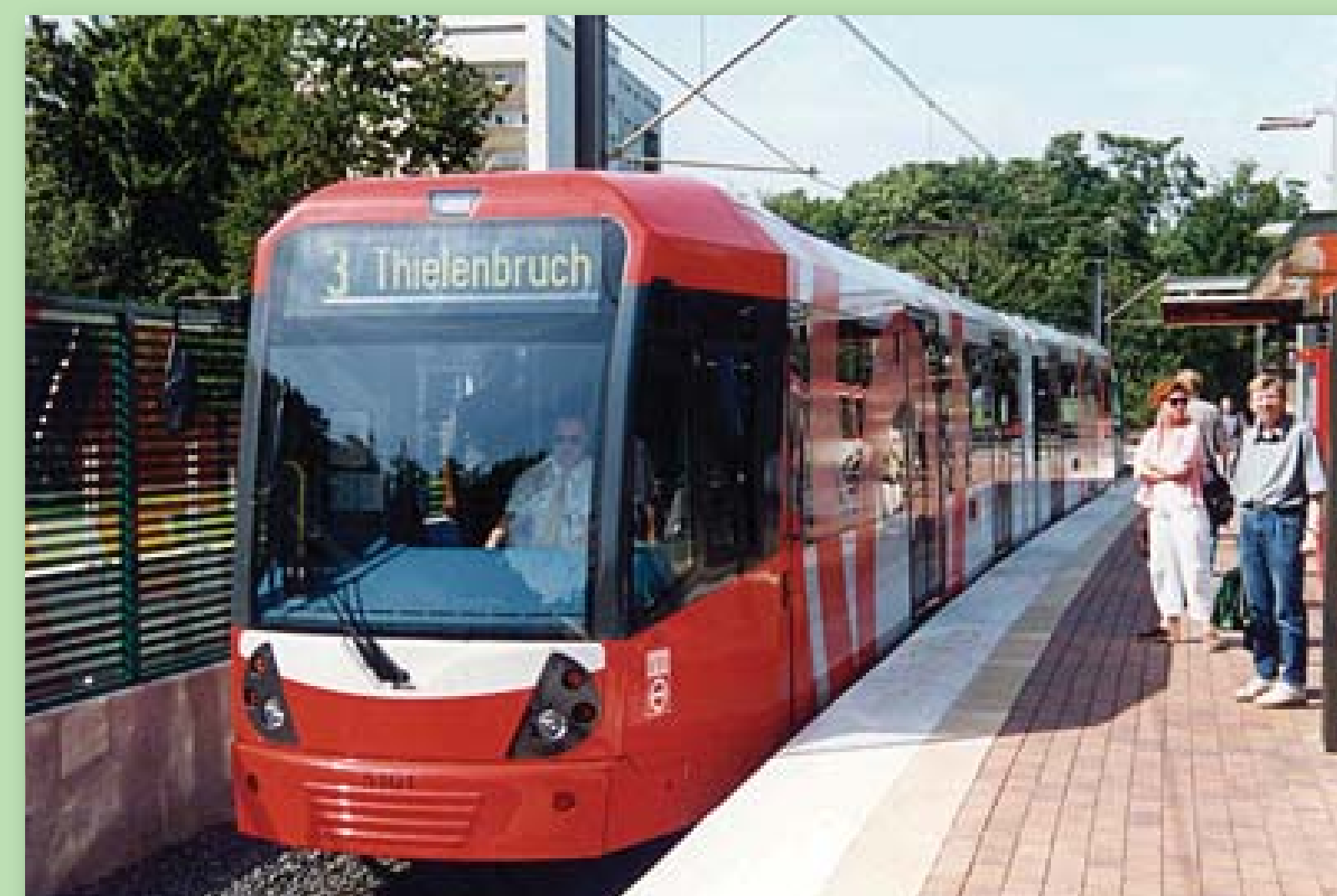
Bombardier Flexity LRT vehicle in Cologne. Source: Bombardier Transportation
